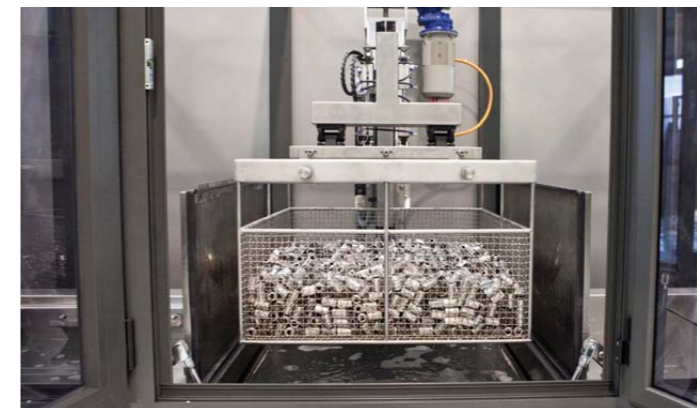
Basket out of tank by rinsing in hot detail. Multi-stage computers can have various types of drying and passivating parts.
