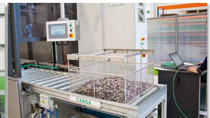
Detail of basket entering ultrasonic station. Racks and baskets are customized according to the needs of customer size.
