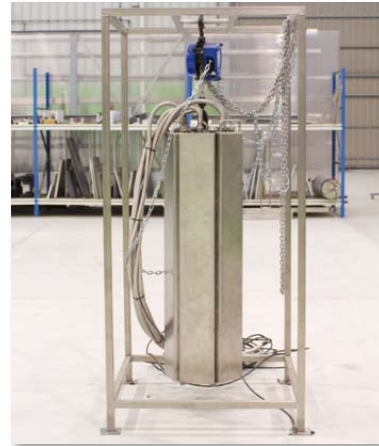
Sets of ultrasonic special application of petroleum industry (large tanks).
